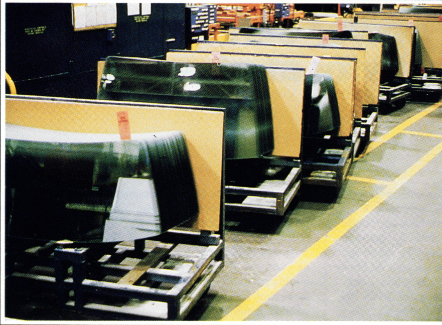
Fig. 4 (above): Staying one shift ahead of the bending lehr, a variety of flat windshield forms wait on wheeled carts. Any downtime in the NC cutter usually requires that a one-shift "cushion" be made up on an overtime basis.
