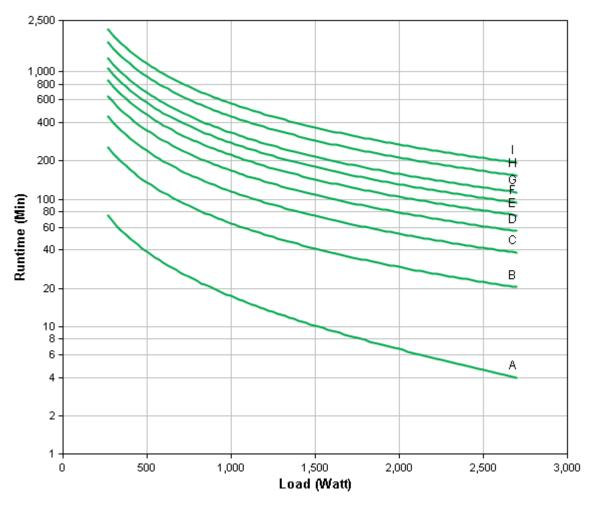
Curve fit to measured runtime data. All measurements taken with new, fully charged batteries, at typical environmental conditions, with no electrical input and balanced resistive load (PF = 1.0) output.
