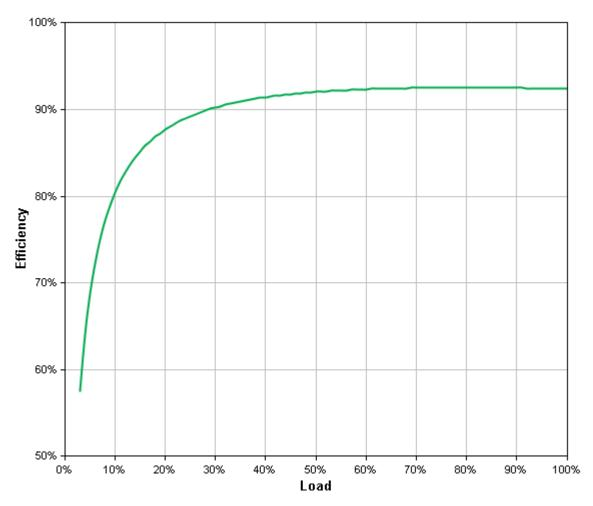
Curve fit of data measured in accordance with the ENERGY STAR Program Requirements Product Specification for Uninterruptible Power Supplies (UPSs) - Eligibility Criteria Version 1.0. All measurements taken in normal mode(s), at typical environmental conditions, with 230V/50Hz electrical input and balanced resistive load (PF = 1.0) output.
